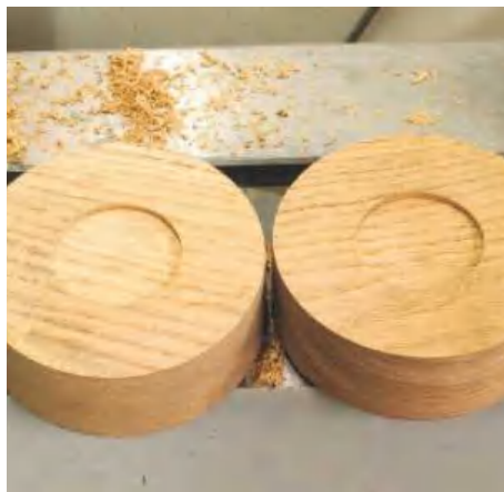
▲ Pic.8 The bottoms of both bases are completed and the diameters are the same. Doing the job in stages means that you don't have to keep swapping between chucks, etc. which makes the process more efficient
